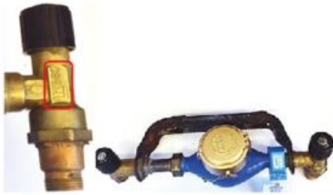
Image of non-approved shut-off valves.
